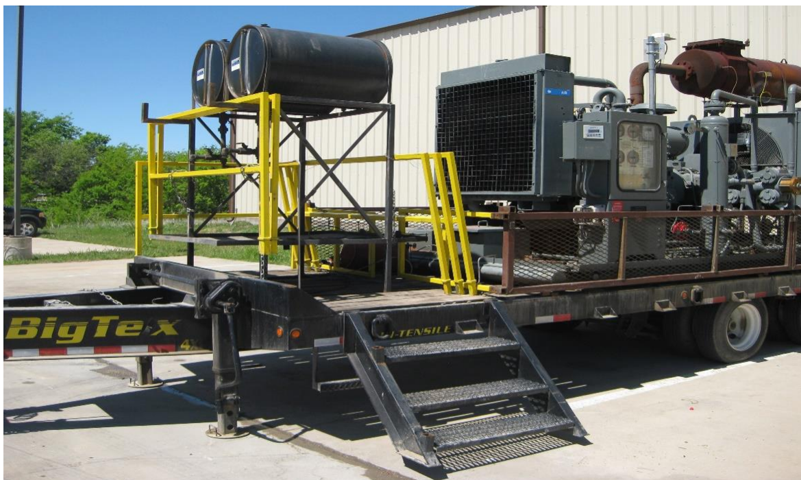
Figure L.13: Trailer-mounted compressor package with accessible oil storage tanks
