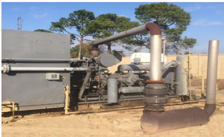
Figure M.5: Silencer placed at ground level to reduce sound travelling over walls at an urban golf course.
