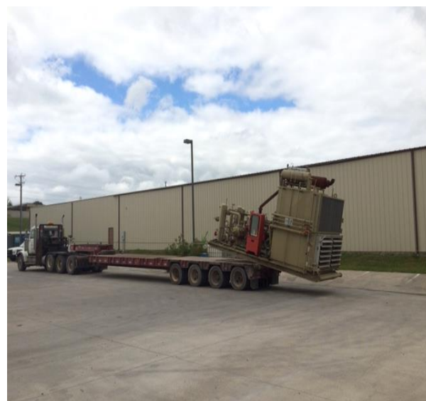
Figure O.3: Complete small compressor package being loaded by tail-boarding.
