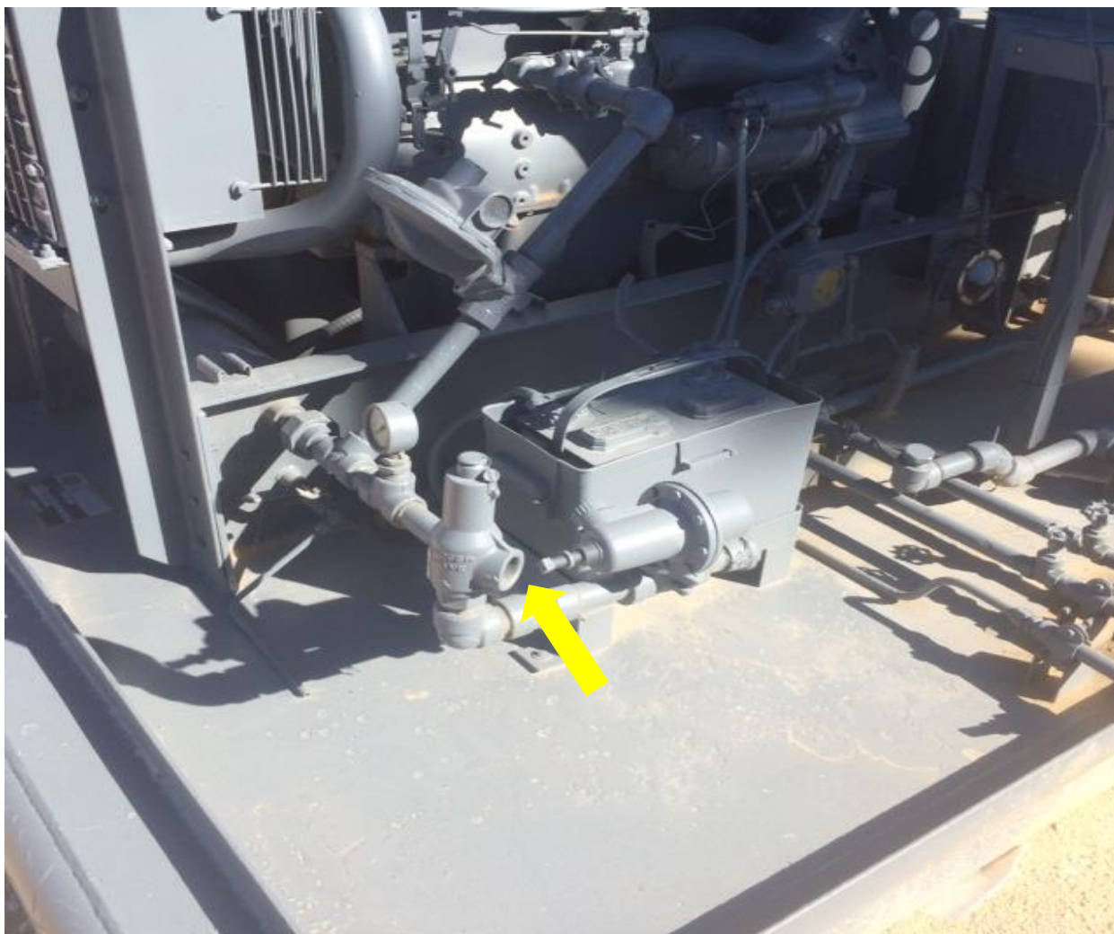
Figure L.12: Example of a poor PSV design that relieves directly at skid level near an open battery box.
