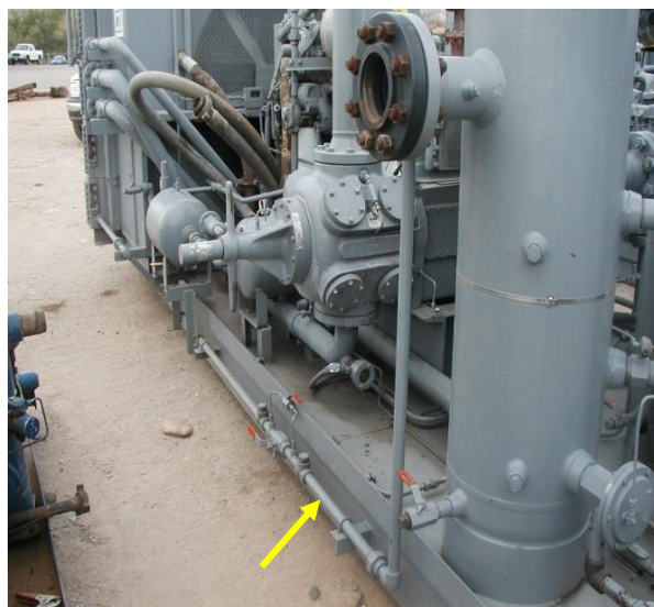
Figure P.7: Small on-skid startup bypass line between compressor discharge and suction.
