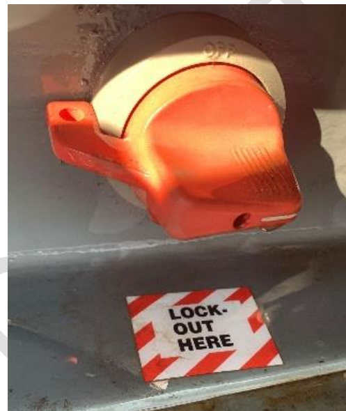
Figure L.10: Example of a battery lock-out device.
