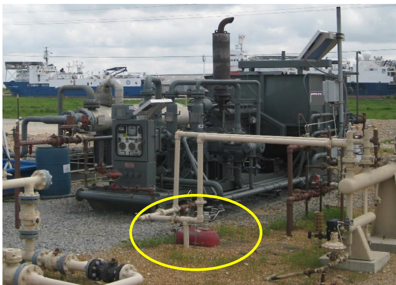
Figure P.18: Off-skid blow case used for collecting liquids from the compressor package.
