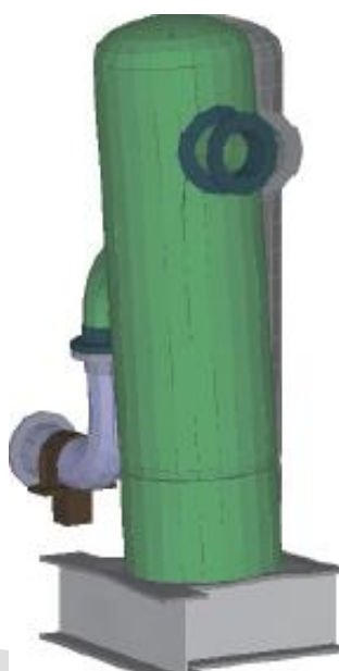
Figure L.17: Exaggerated example of scrubber vibration
