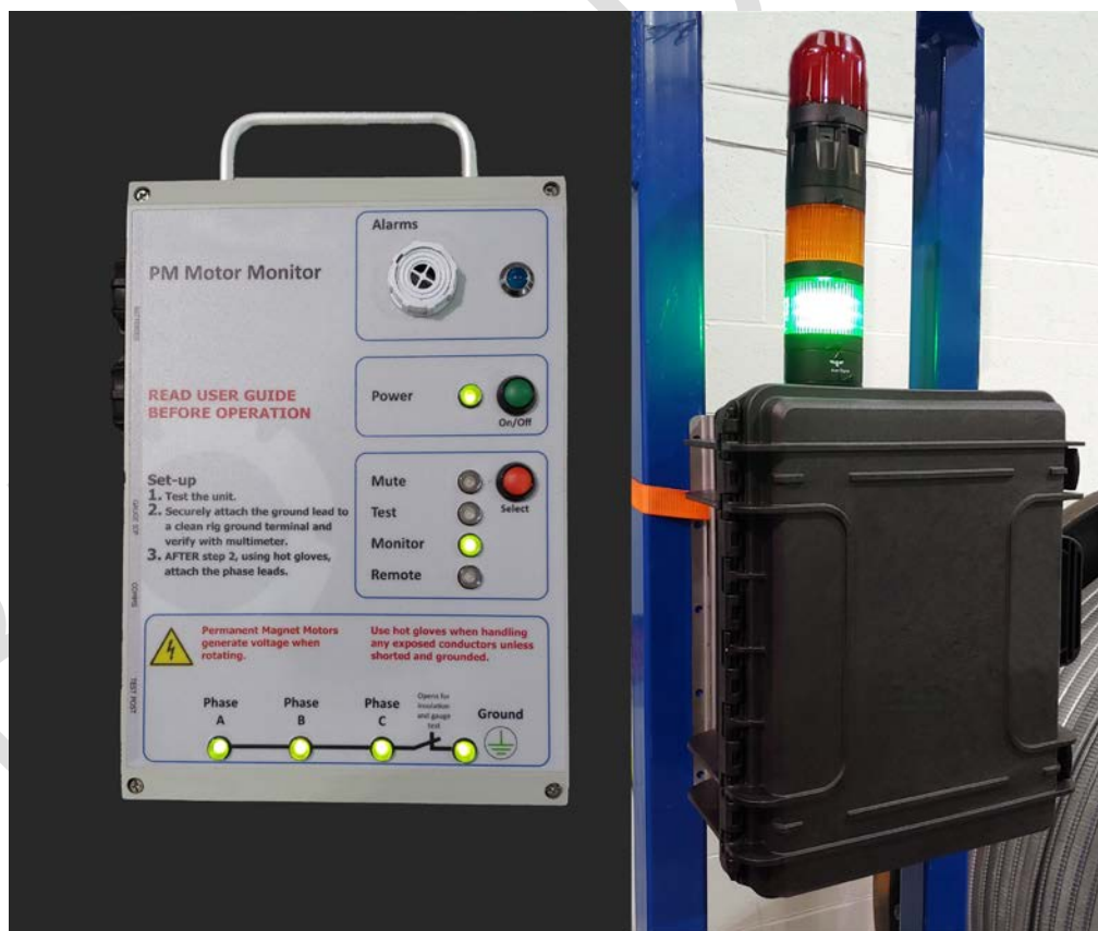
Figure K.5—Continuous monitoring shorting and grounding for spooler and splicing.
