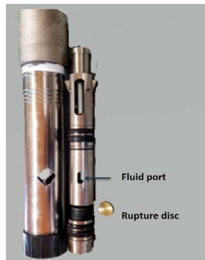
b) wireline insert with rupture disc
