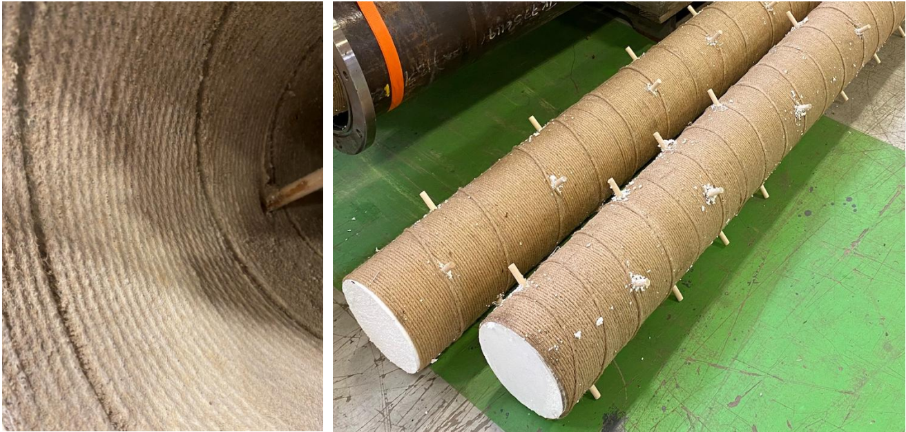
Figure D.2—Illustration of Open Hole Test Fixture and Internal Profile
