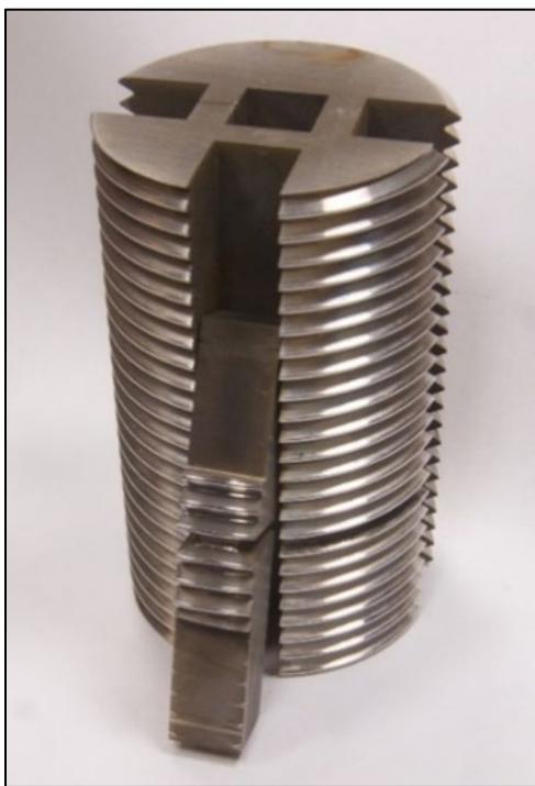
Figure 1—Example of specimen extraction locations from threaded product
