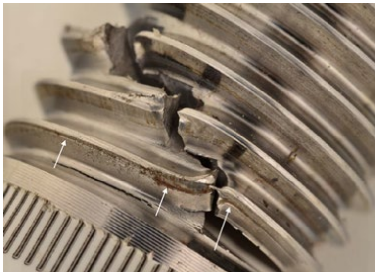
Figure 2—1-in. Bolt,1-D-M-U-7, Showing an Imperfection in the thread flank (white arrows)
