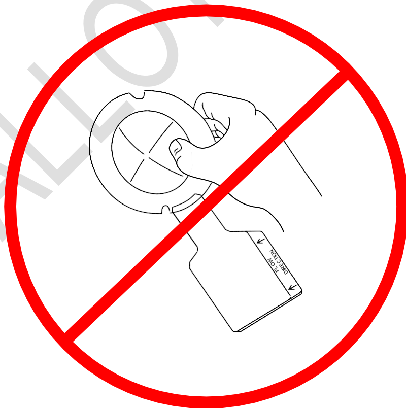
Figure A.2—Proper Handling of a Rupture Disk
