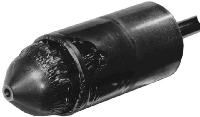
Figure 12—Flashing Damage
