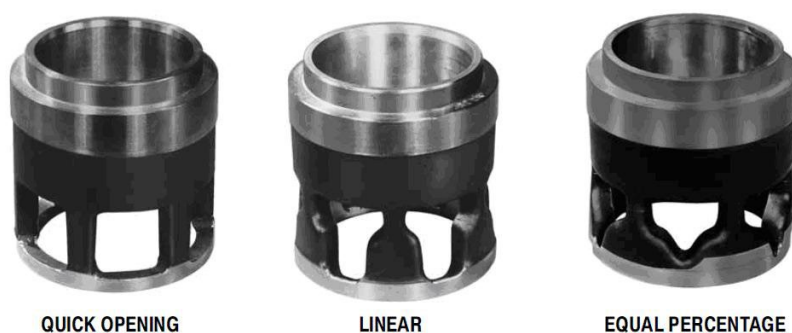
Figure 5—Characterized Cages for Globe-style Valve Bodies
