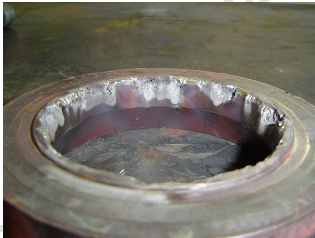
Figure 10B—Cavitation Damage to Seal Ring
