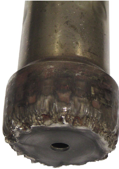
Figure 10A—Cavitation Damage to Valve Plug
