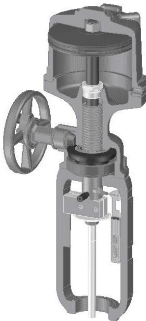
Figure 21—Side-mounted Handwheel
