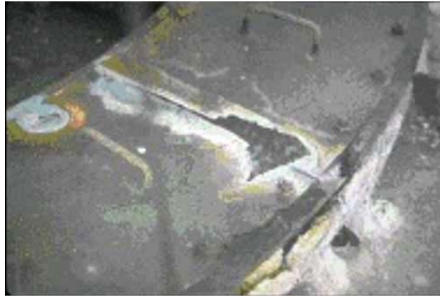
Figure 18—Dew Point Corrosion from Flue Gas Corrosion on Radiant Section Header Box
