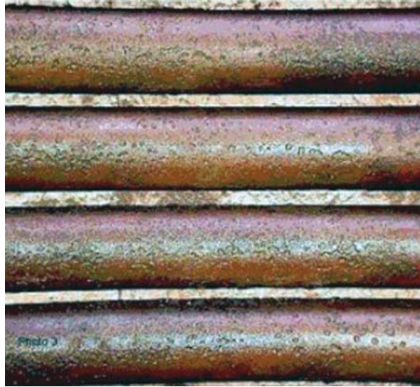
Figure 11—General Metal Loss and Pitting of Tubes Exposed to Moisture and Corrosive Deposits During Idle Periods
