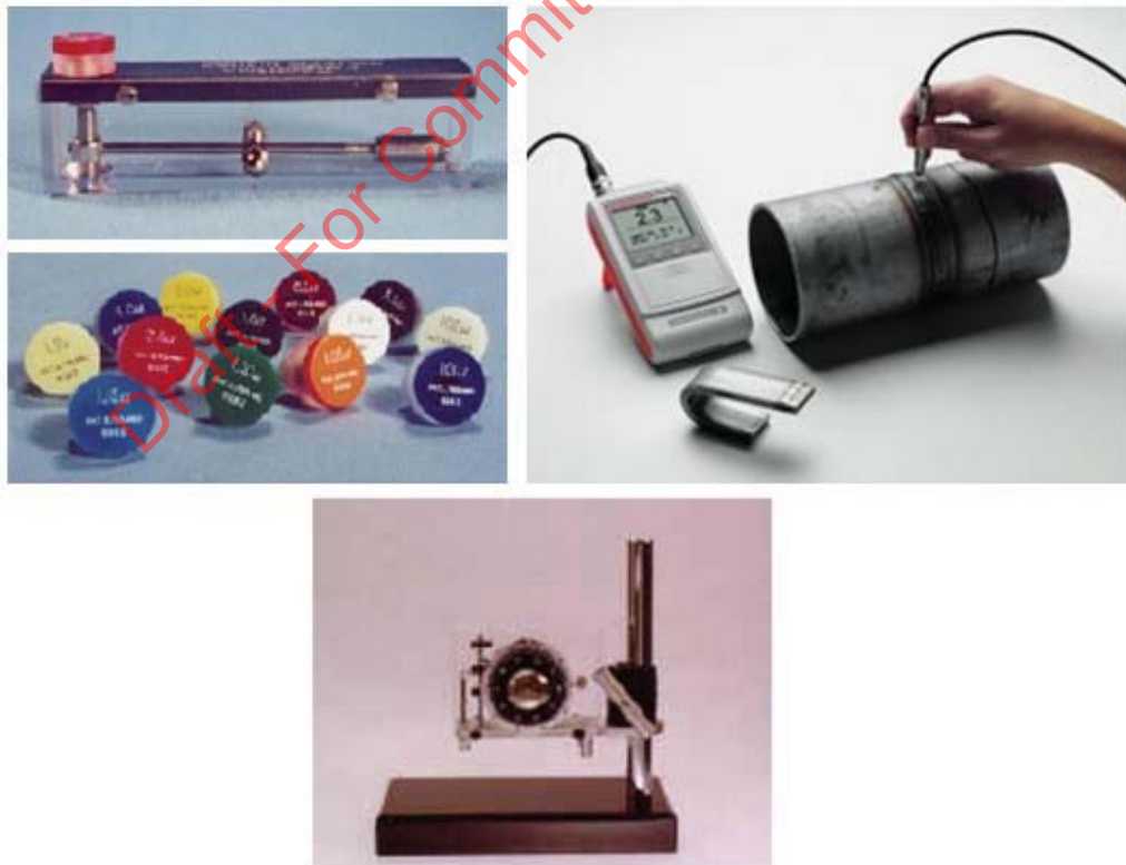
Figure 33—Various Magnetic Measurement Devices (Clockwise from Top Left: Severn Gauge, Feritscope, and Magne Gauge)
