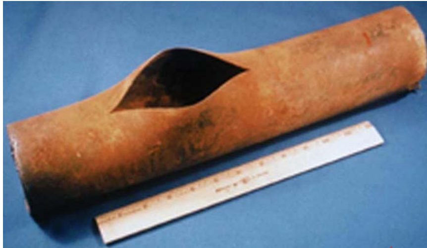
Figure 20—Bulged and Split Tube
