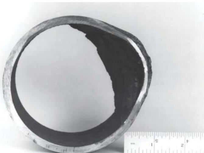
Figure 16—Short-term Boiler Tube Failure Caused by Waterside Deposits, Subsequent Overheating, and Final Bulging of the Tube Wall
