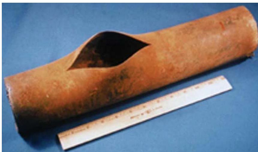
Figure 20—Bulged and Split Tube
