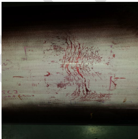
Figure 7: - Two examples of ECSSC detected with PT
