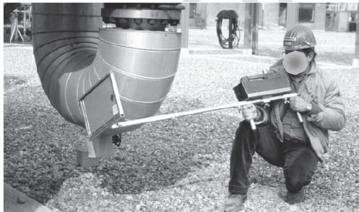
Figure 811 18—Photo of a Flash Radiography System for Pipe Profiling to Detect Wall Thinning Due to Corrosion
