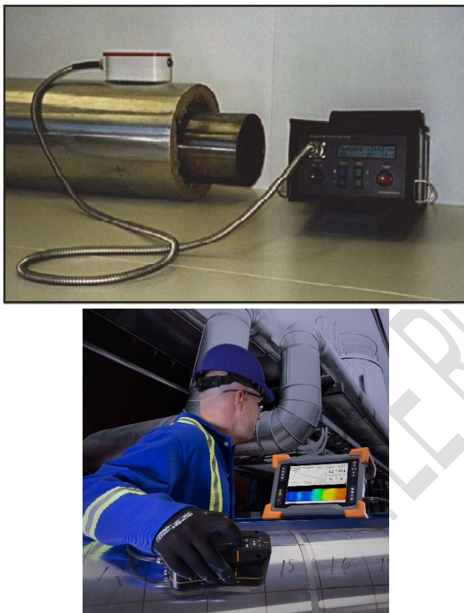
Figure D.3—A Pulsed Eddy Current Instrument with Probe and being used during an examination.
