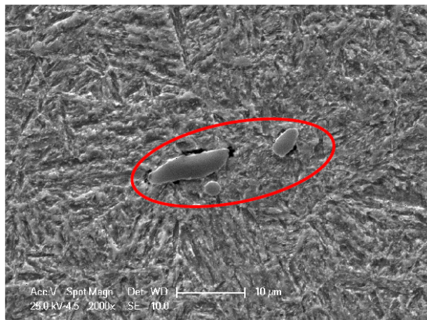
Figure 7—Larger Size and Higher Density of MnS Inclusions in AISI 4340 Material Analyzed
