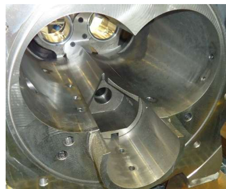
Figure C.7 – Oil-flooded Slide Valve Showing Radial v_i Cutout
