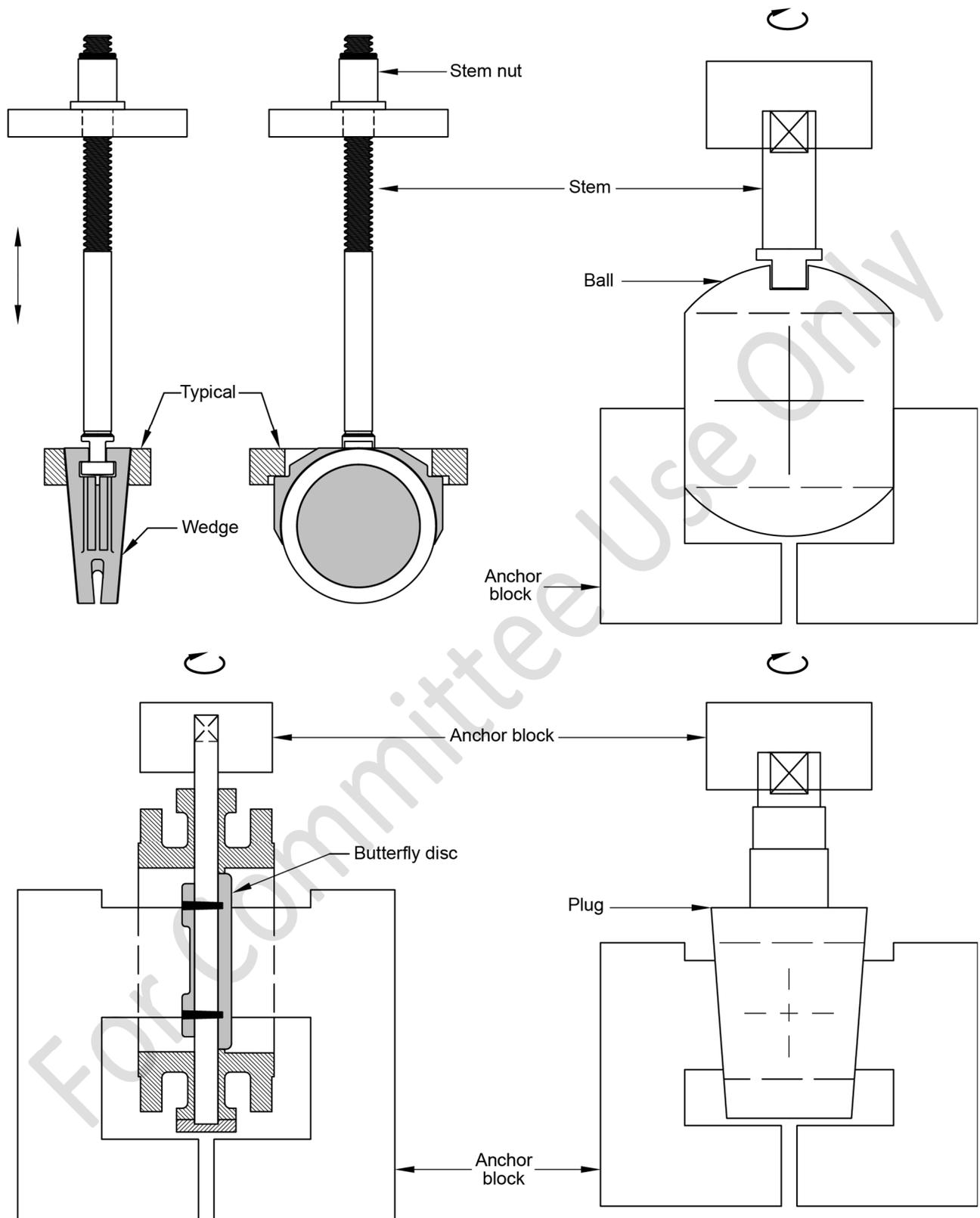
NOTE Diagrams shown are only examples of allowed fixtures for strength testing.
