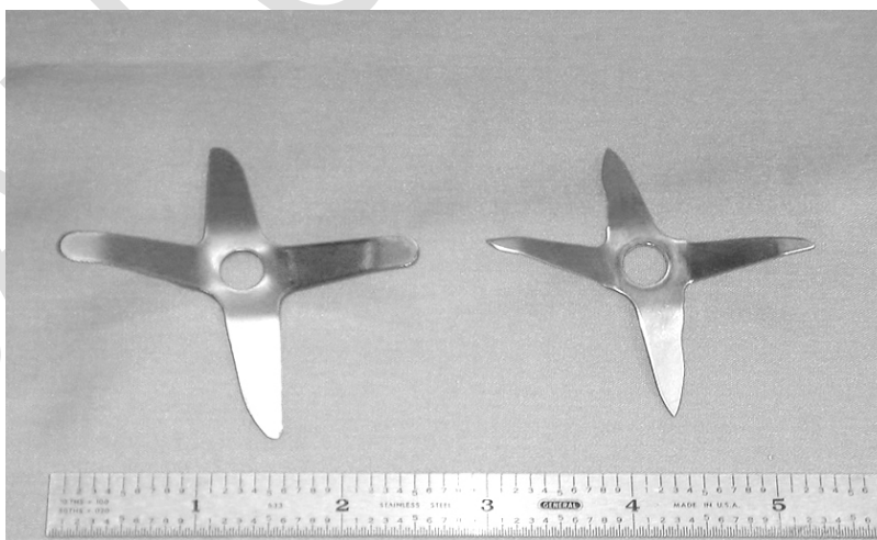
Figure B.1—Worn Blade (right) Compared to a New One (left)
