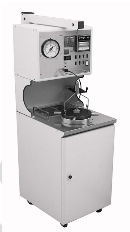
Figure 4—Typical Pressurized Consistometer
