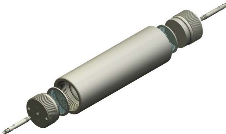
Figure 10—Common Screwed-cap Type, HPHT, Double-ended Fluid-loss Cell
