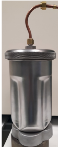
Figure G.1—Example of De-airing Mixing Container
