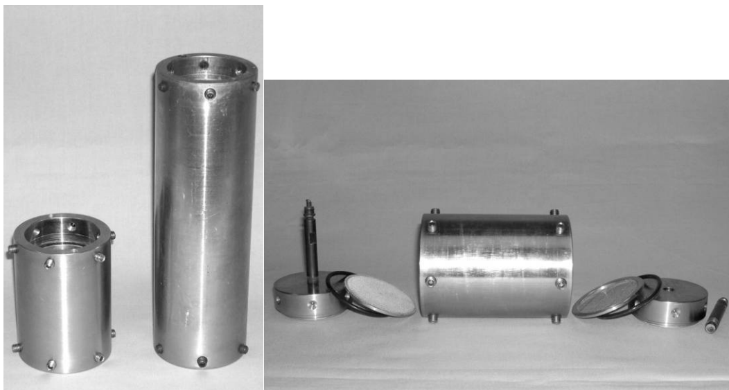
Figure 9—Common HPHT, Non-stirred Fluid-loss Cell Bodies
