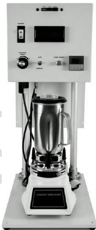
Figure 2—Example of a Typical Cement mixing Device
