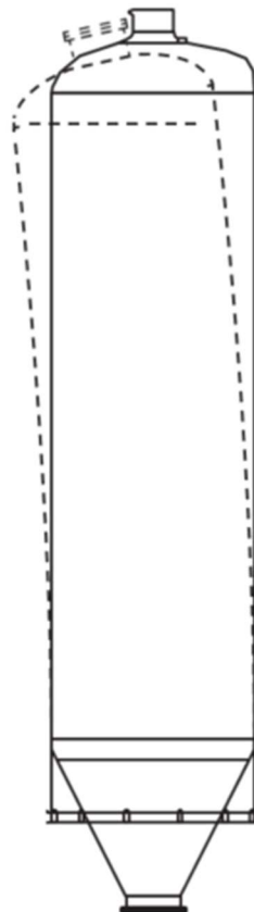
Figure 1 - Bent Drum in a Delayed Coking Unit
