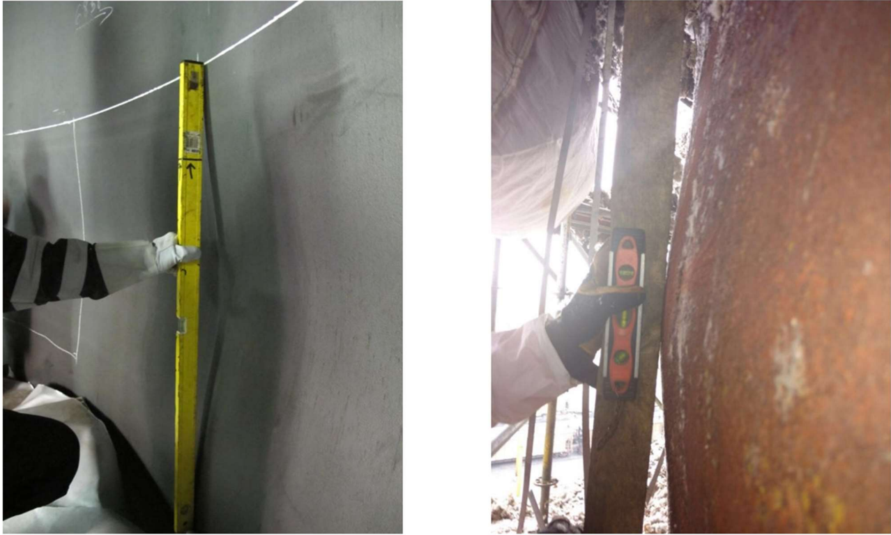
Figure 32—Use of a Straight Edge from the ID and OD to Measure Bulging
