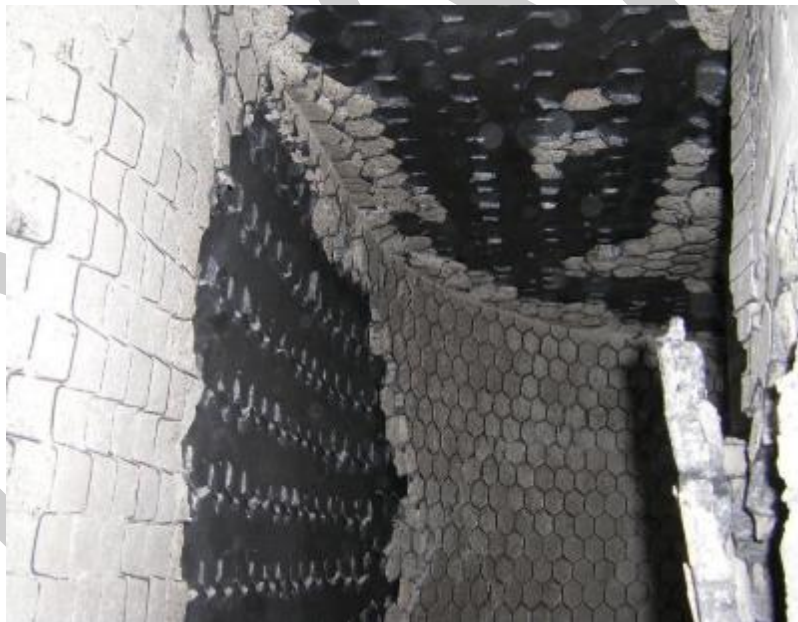
Figure B.20– Corrosion of Hex Attachment Welds
