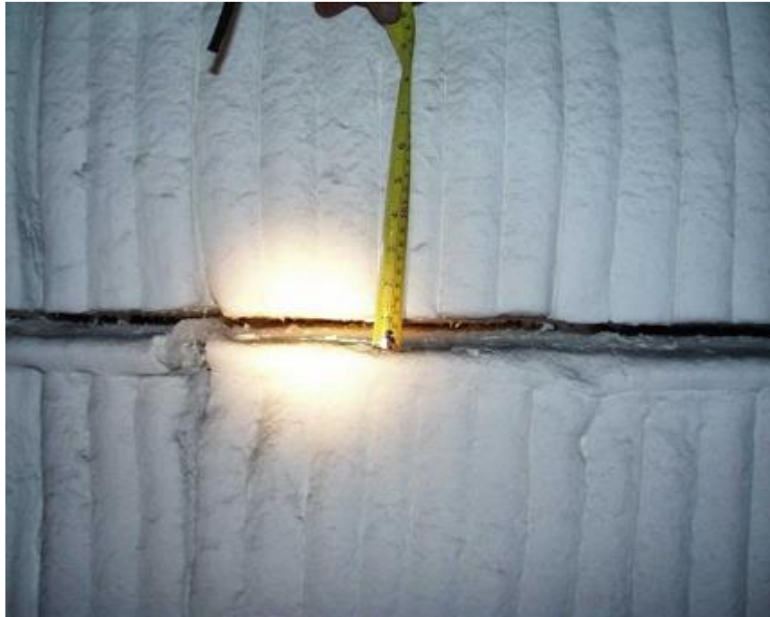
Figure B.12 – Excessive Shrinkage of Ceramic Fiber Modules
