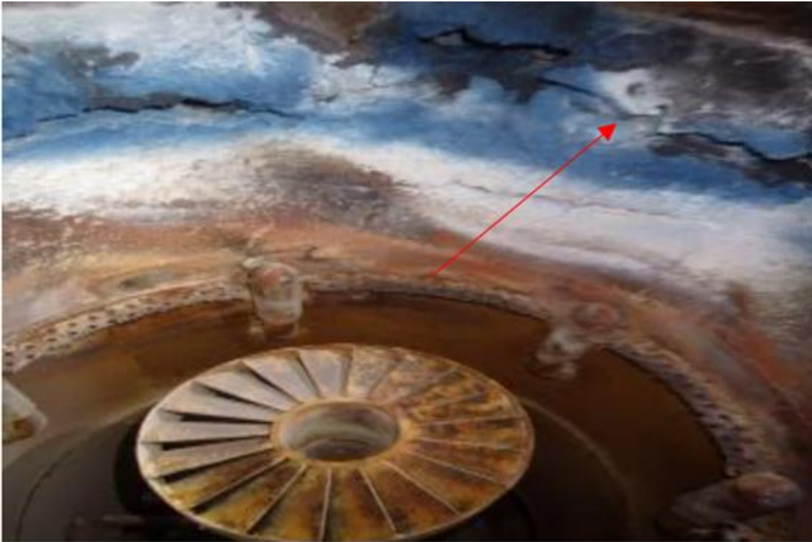
Figure B.14– Overheating and Cracking from Flame Impingement
