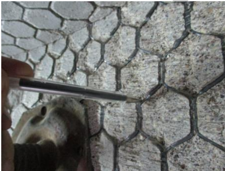
Figure B.1 – Erosion of Hexmetal in FCCU Regenerator Cyclone Caused by High Velocity Catalyst
