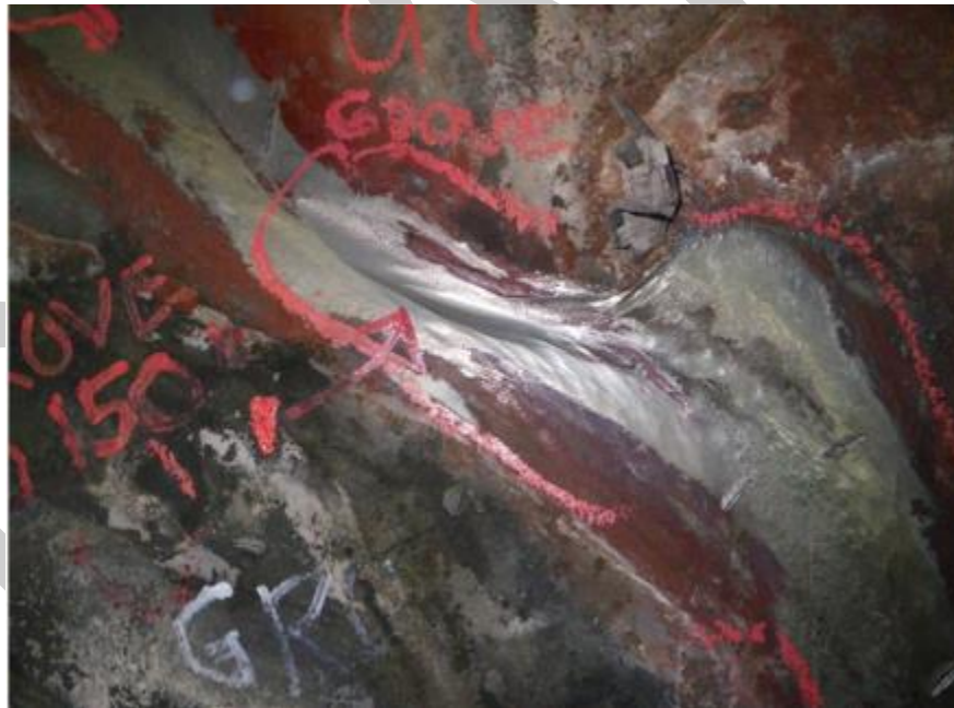
Figure B.24– Shell Erosion Caused by Hot Gas Bypass
