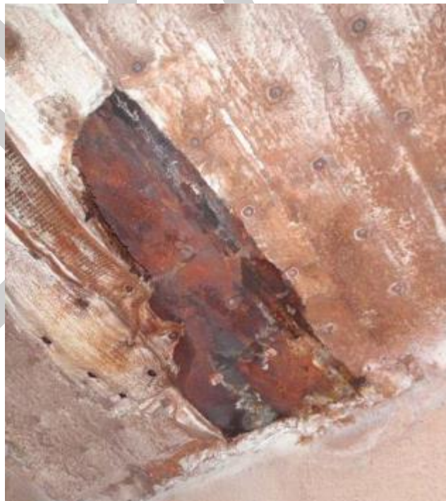
Figure B.18- Dew Point Corrosion of Shell and Anchors
