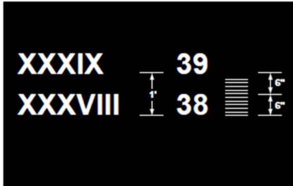
Figure B-5—Draft Readings: US Customary Unit
