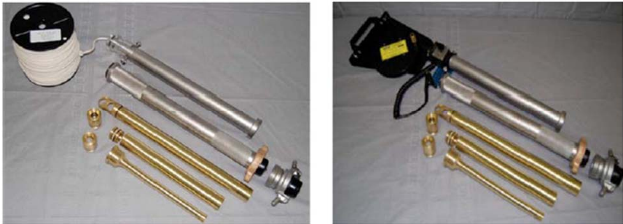
Examples of Typical Special Weighted Bar and Bob Units
