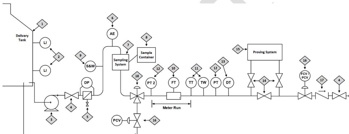
Figure 1 – Typical LACT Metering System
