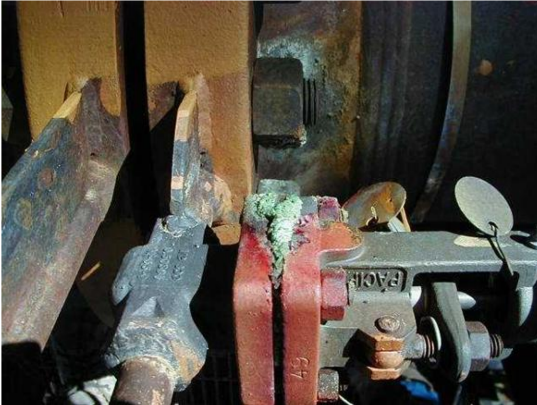
Figure E.2—Example of Category 2 Leak
