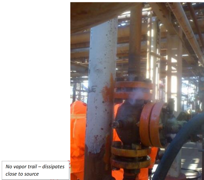
Figure E.3— Example of Category 3 Leak
