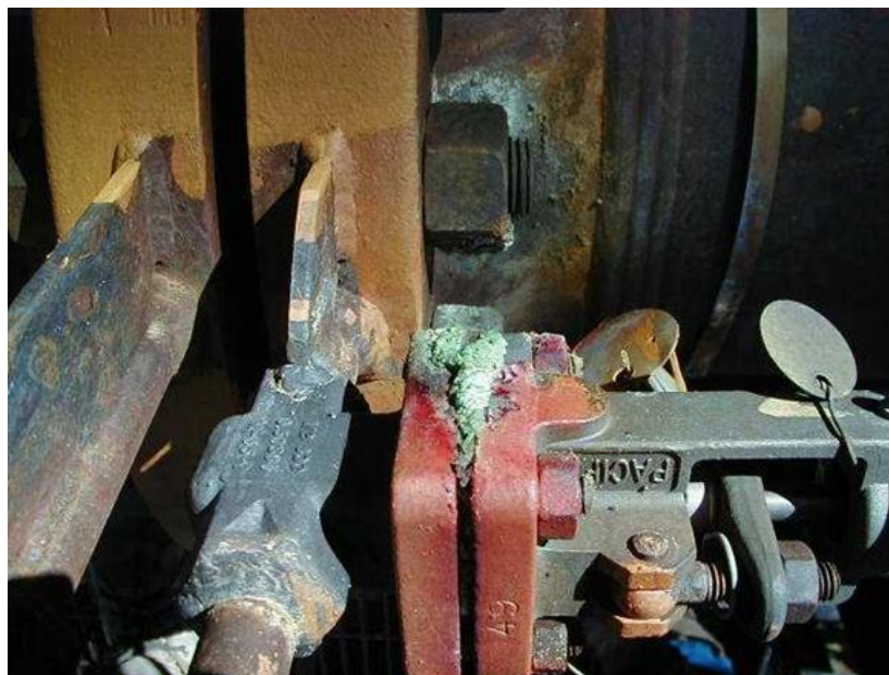
Figure E.2—Example of Category 2 Leak
