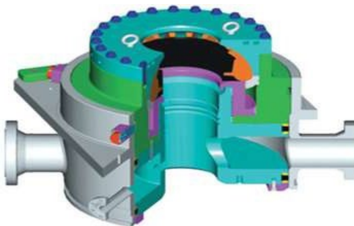
Figure 1—Example Diverter with an Annular Packing Unit
