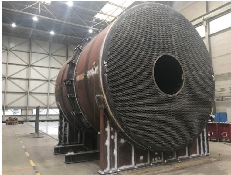
Figure 39—Regenerator heat exchanger with Grade 91 steel shell
