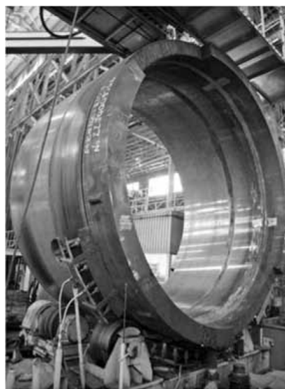
Figure 38—Mock-up with a wall thickness of 225 mm (forged ring), comprising one circumferential seam and one nozzle weld
