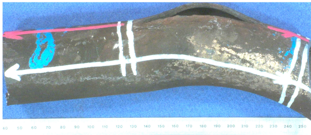
Figure 26—Grade 91 steel boiler superheater tube (T91) that failed due to overheating in 4 years
