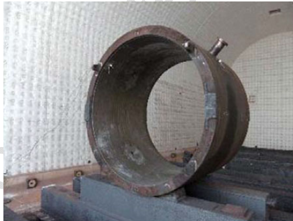
Figure 37—Completed mock-up with a wall thickness of 160 mm, comprising four longitudinal weld seams and three nozzle welds
