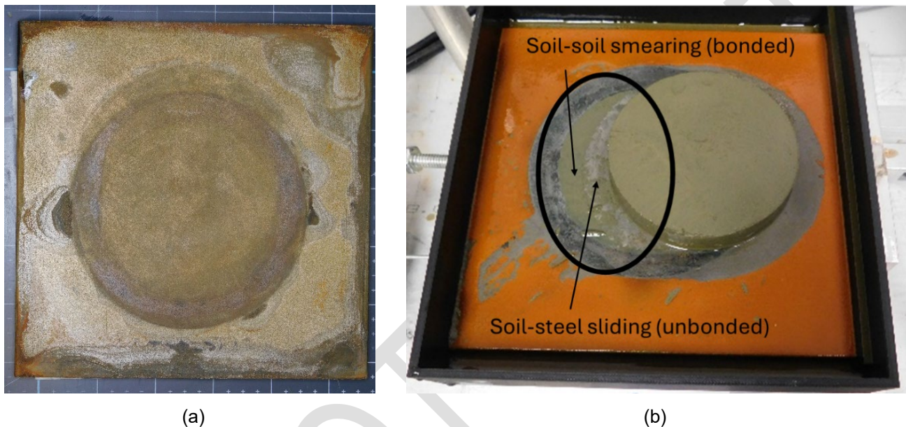
Figure 46 – Pre-test and post-test images of bare steel surface test showing (a) rust developing between tests and (b) changes in bonding between the soil and the surface during shear (Das et al. 2024)
