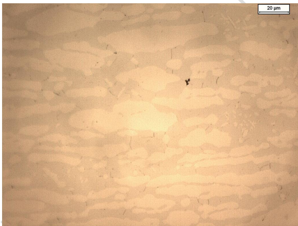
Figure I.1—Just acceptable microstructure: Discrete/standalone intermetallic precipitates not greater than 10 μm (0.40 mil). Electrolytic etching using 10 % NaOH
