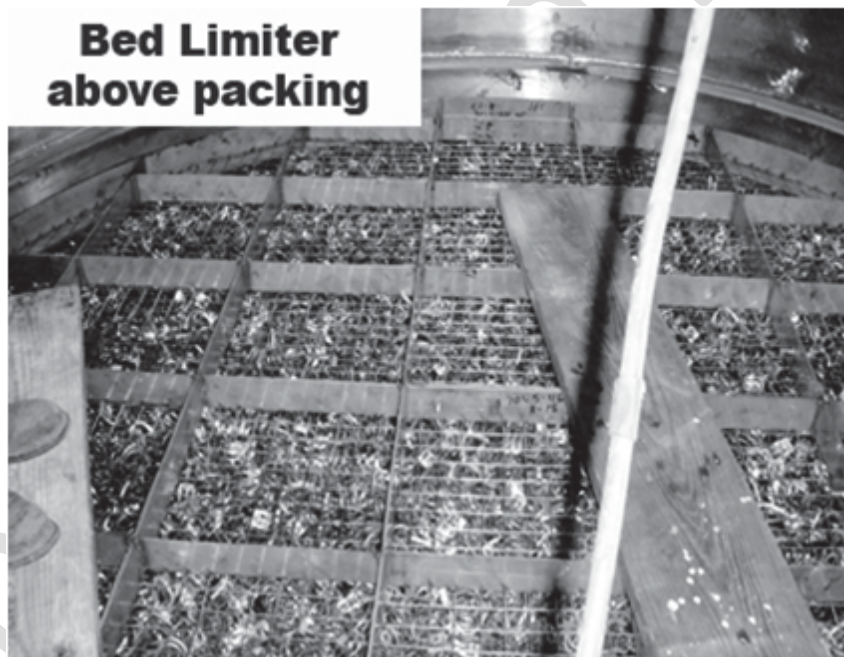
Figure B.43 - Bed Limiter Above Random Packing
