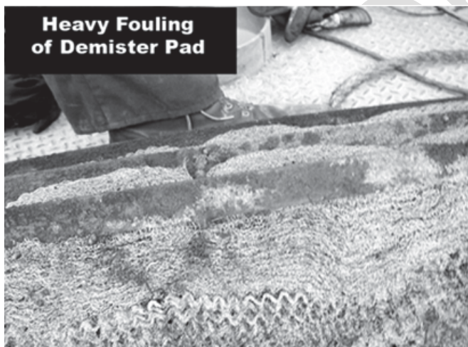
Figure B.31 - Fouled Demister Pads
