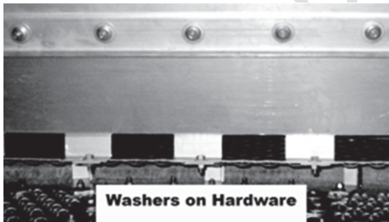
Figure B.41 - Hit the Washers, Not the Bolts
