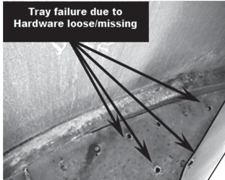
Figure B.78 - Loose and Missing Hardware Failure
