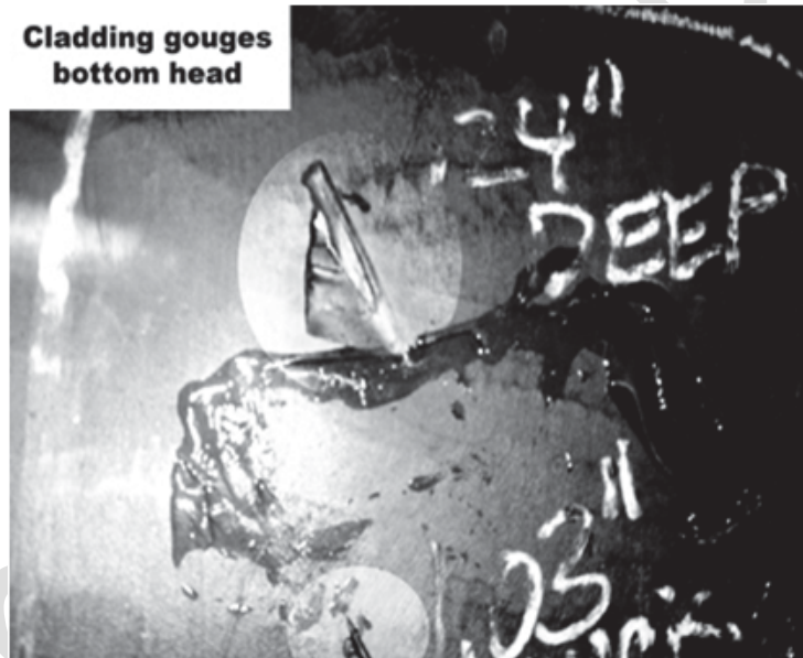
Figure B.52 - Cladding Breach at Gouges in Bottom Head
