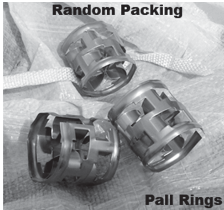
Figure B.13 - Random Packing, Pall Rings
