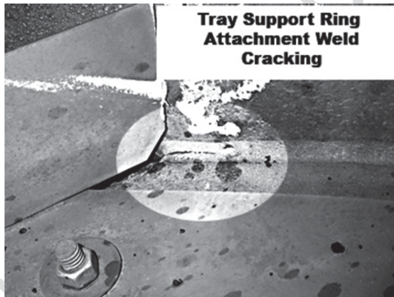
Figure B.85 - Cracking of Ring Attachment Weld
