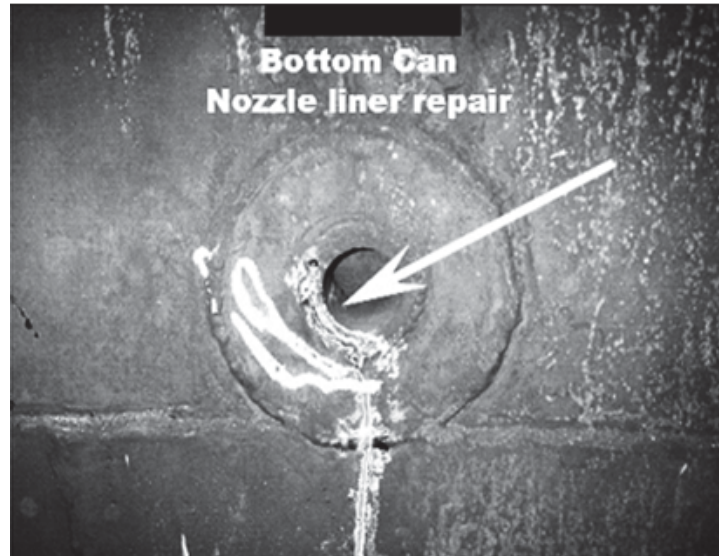
Figure B.51 - Stainless Steel Donut Cladding Breech
