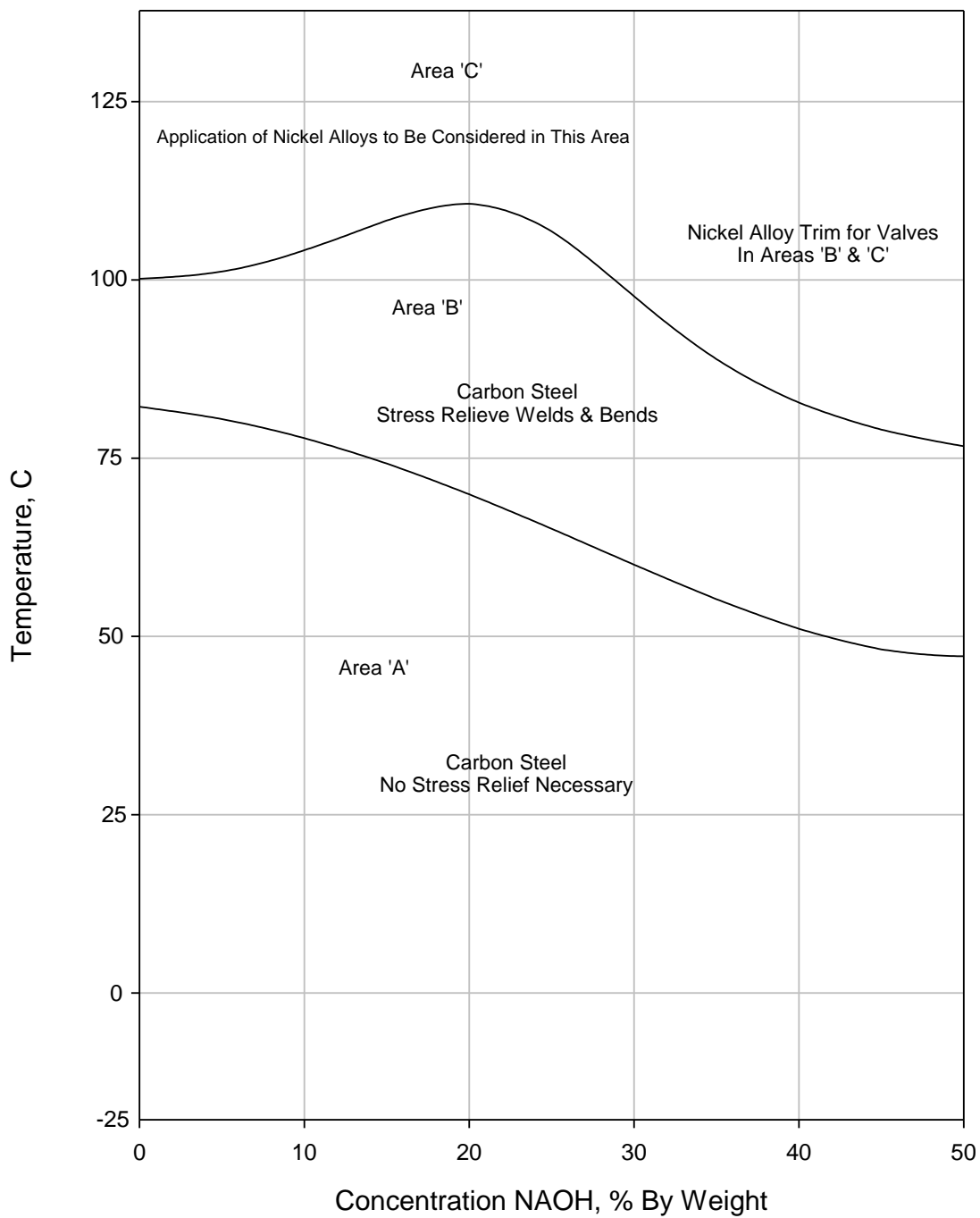
Figure 2.C.4.1M—Susceptibility of Caustic Cracking in Carbon Steel
