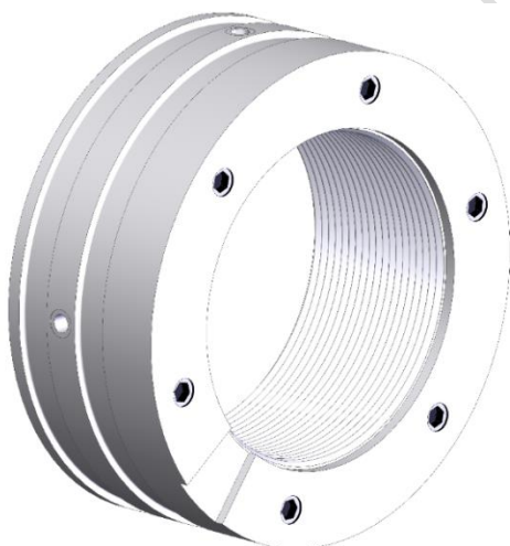
Figure 78—Ring Gauge with Step Plate
