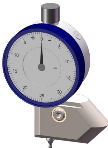
Figure 46—Example Thread Height Gauge for Internal / External Buttress Threads
