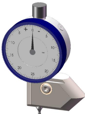
Figure 52—Example of Addendum Gauge-Balanced Indicator
