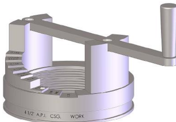
Figure 79—Step-type Ring Gauge
