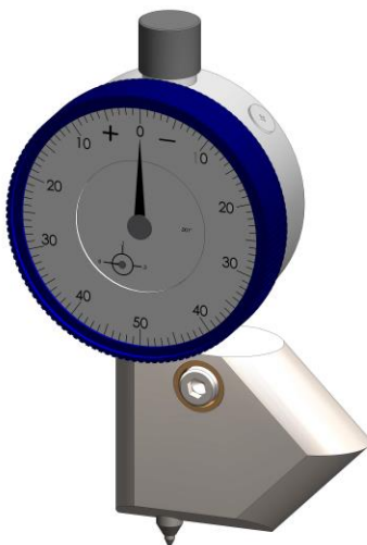
Figure 44—Thread Height Gauge for Internal / External Threads—Balanced Indicator
