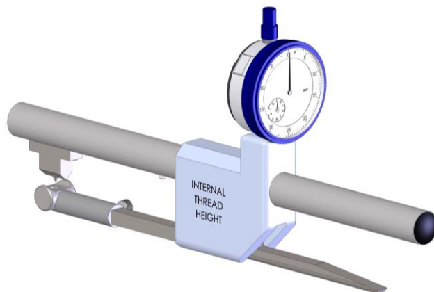
Figure 45—Thread Height Gauge for Internal Threads
