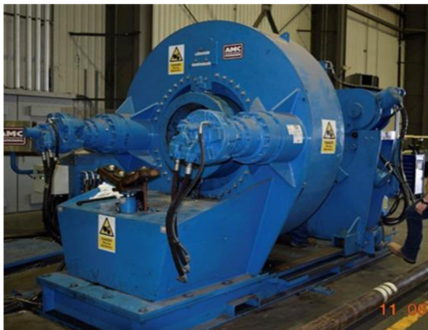
Figure 13—Bucking Unit with Torque of 200,000 ft-lb
