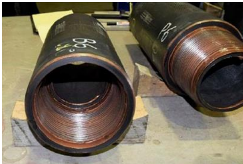
Figure 23—6-5/8 FHDS Box B6 after Break-in Cycle Make-up
