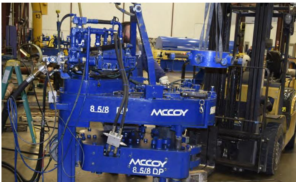
Figure 4—Tongs Used to Conduct Torsion Tests on NC50DS Connections
