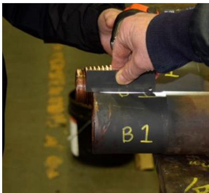
Figure 20—NC26DS Pin P2 after Make-up to 14,070 ft-lb in Torque-to-failure Test
