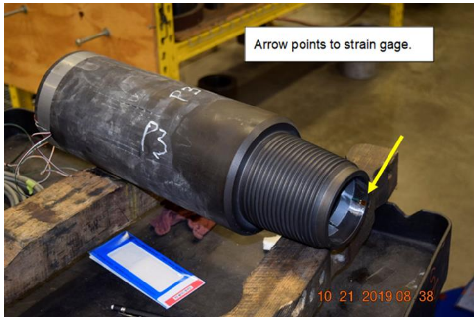
Figure 11—NC50DS Pin P3 for Torque-to-yield Test
