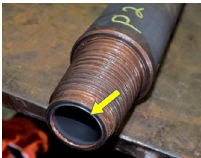
Figure 20—NC26DS Pin P2 after Make-up to 14,070 ft-lb in Torque-to-failure Test
